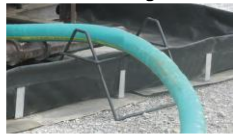
Steel Hose Bridges
